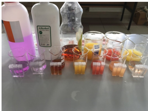
Figure 3: The experiment in progress when the solvents are in the beaker and pomegranate stained filter paper are put in.
