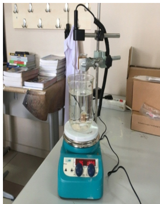
Figure 3 The hot plate is arranged to 25 °C, and a test tube is immersed into the water by an extension clamp
