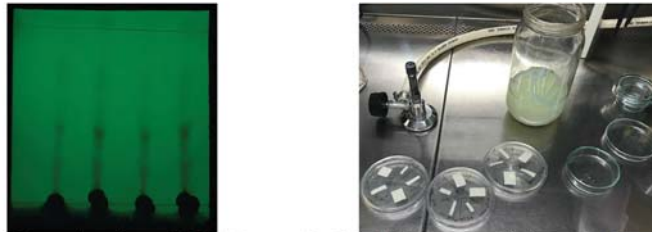
Figure 11: 1. Examination of TLC Paper Under 312 nm Irradiation 2. Using the Separated Materials in Antibigram Test
