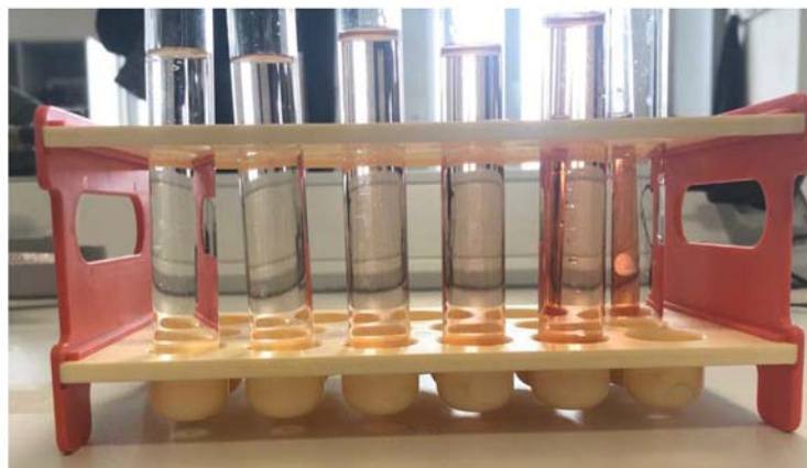
Figure 4.2: [\text{Fe}(\text{SCN})_6]^{3-} standard solutions lower to a higher concentration. (from left to right)
