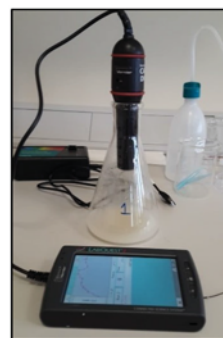
Figure 4: Maintaining the yeast activity using Vernier CO 2 probe.
